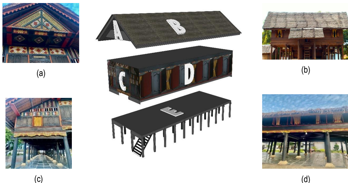
Figure 2. Decomposition of plane structures in the construction of Rumoh Aceh
